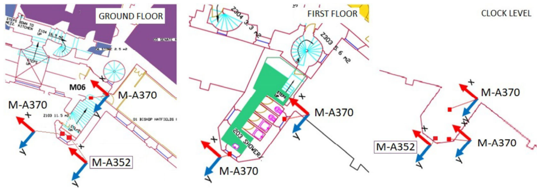
Figure 15. Adopted sensor layout at the clock tower during the ambient vibration campaign. M-A352 accelerometers were installed at the ground floor and at the clock level of the tower.
