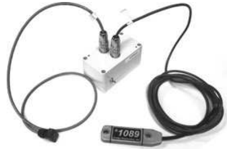
Fig. 1. Wireless sensor system (WSS) node with accelerometer and strain transducer.
