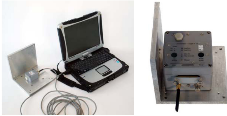
Fig. 1. USB Acceleration sensor with laptop (left) and wireless LAN acceleration sensor (right).
