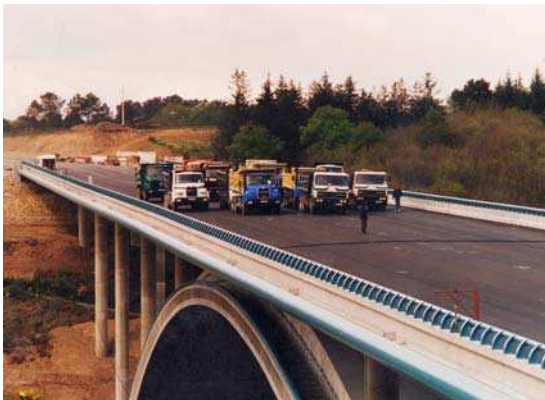
Figure 12: Loading of an arch bridge.
