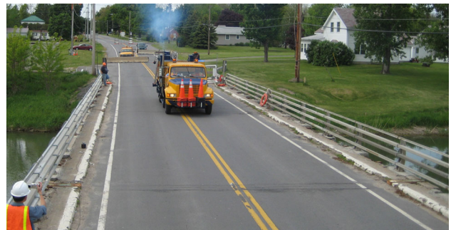
Fig. 4 Photograph of instrumented bridge span and vehicle used for controlled application of test loads
